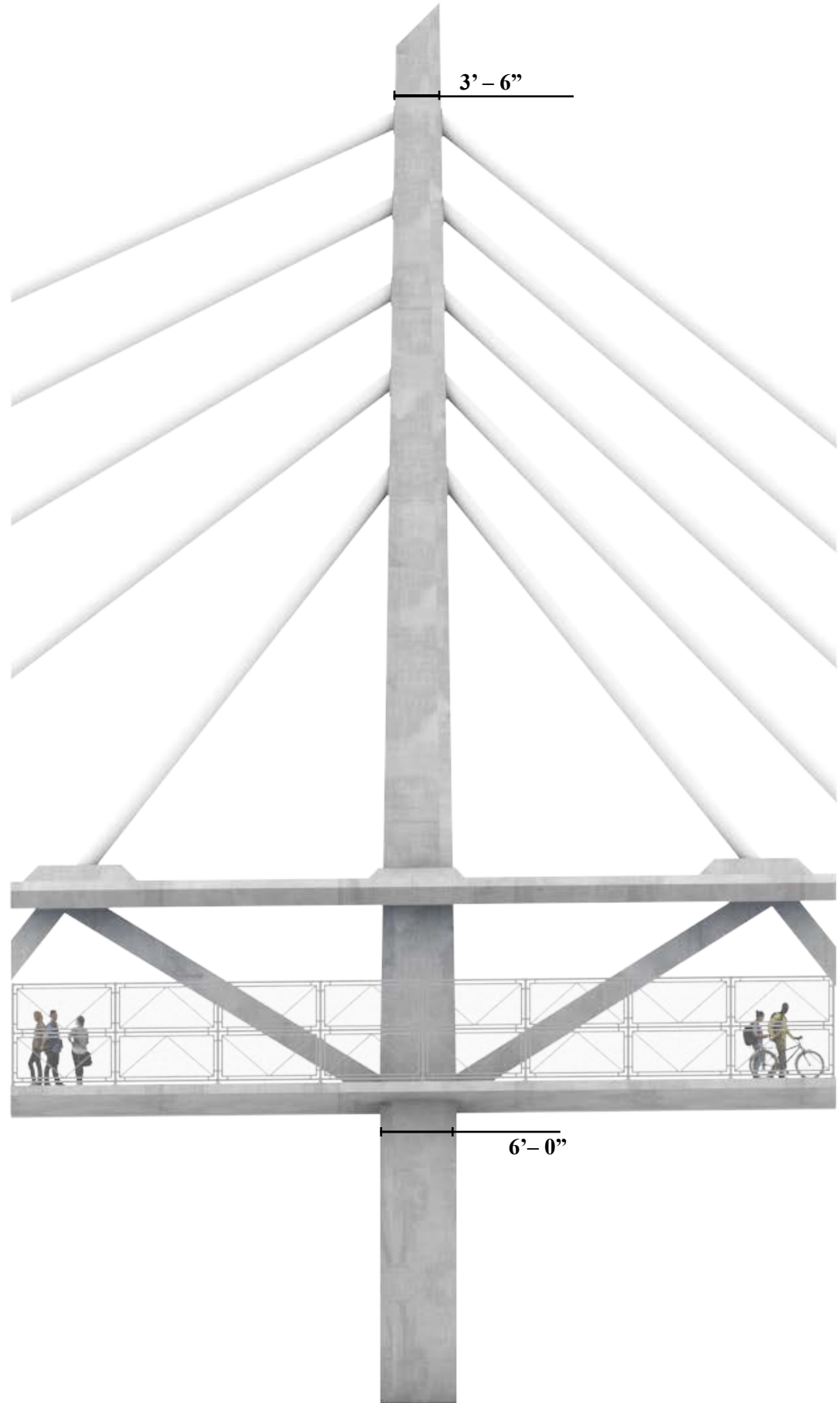
5 Sets of stays in a fan arrangement
